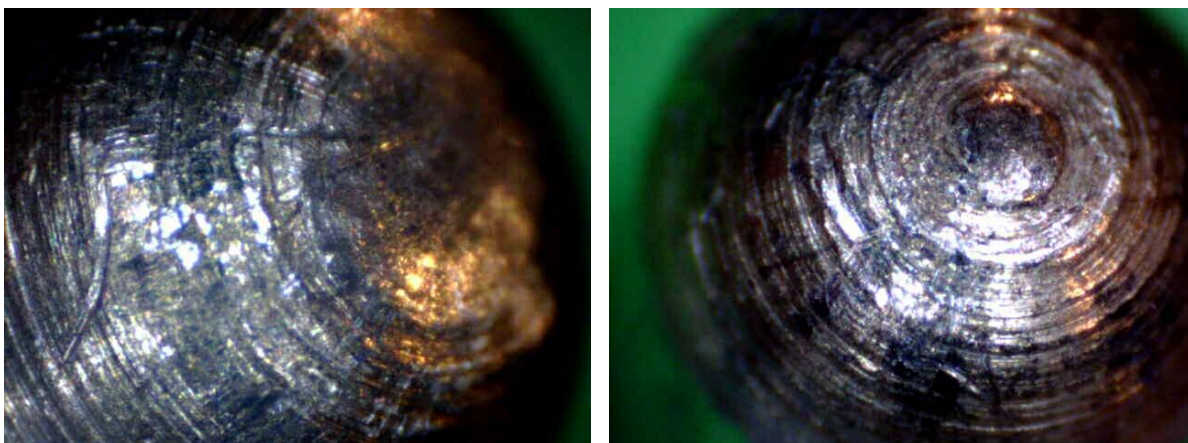
Figure 3.2: Tool mark evidence left by a carbon fiber lockpicking tool from a lock that was picked one time. Notice the light scratches and polishes made on the bottom of the pins.
