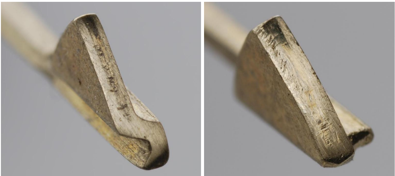
Figure 4.10: The tips of two of the Tricerapick tools showing surface deformities and wear.
