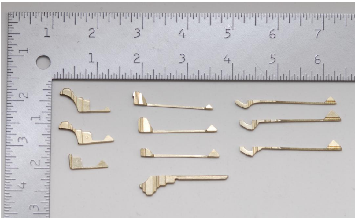
Figure 4.1: The Tricerapick lockpicking set (first edition, 10 pieces)
