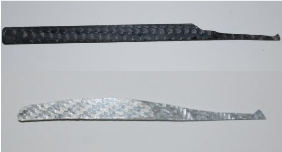
Figure 3.1: Working examples of carbon fiber (top) and fiberglass (bottom) lockpicking tools.
