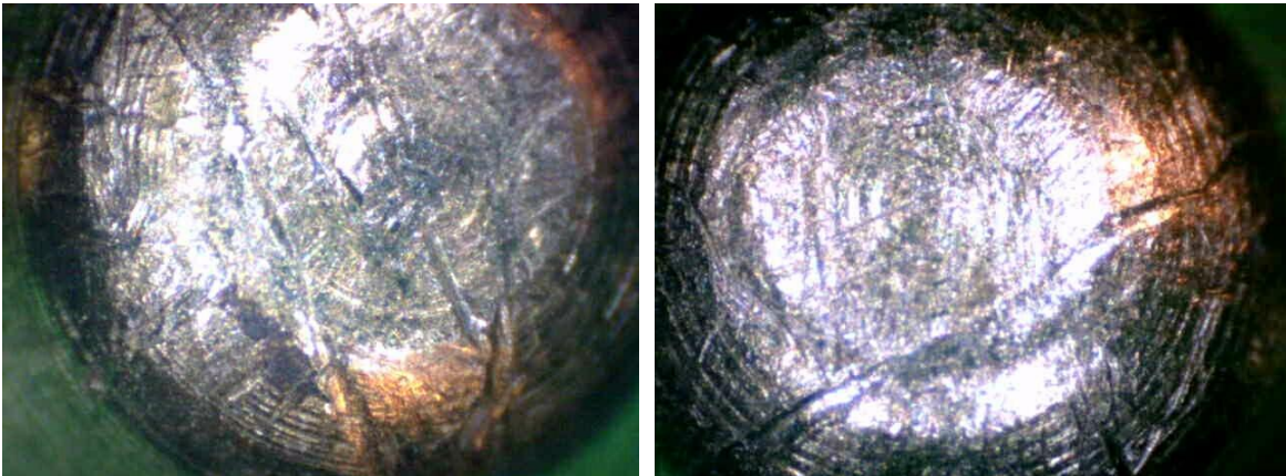
Figure 2.1: Tool marks from the pin-tumblers of a lock picked once with steel tools.
