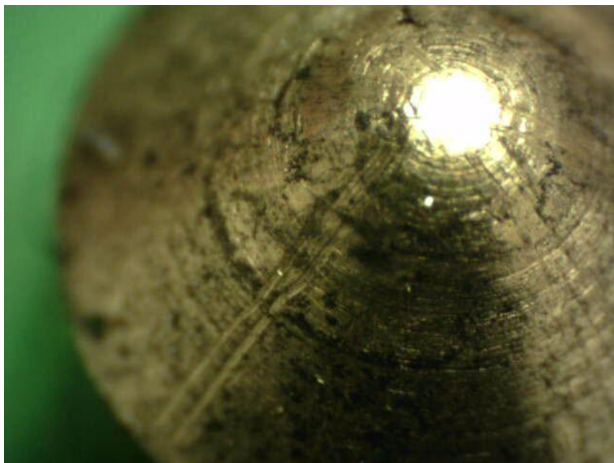
Figure 4.5: A distinct key track, caused by the Tricerapick. In addition to being quite deep in the brass, there is a slight wave in the center of the tool mark; something atypical of normal wear.
